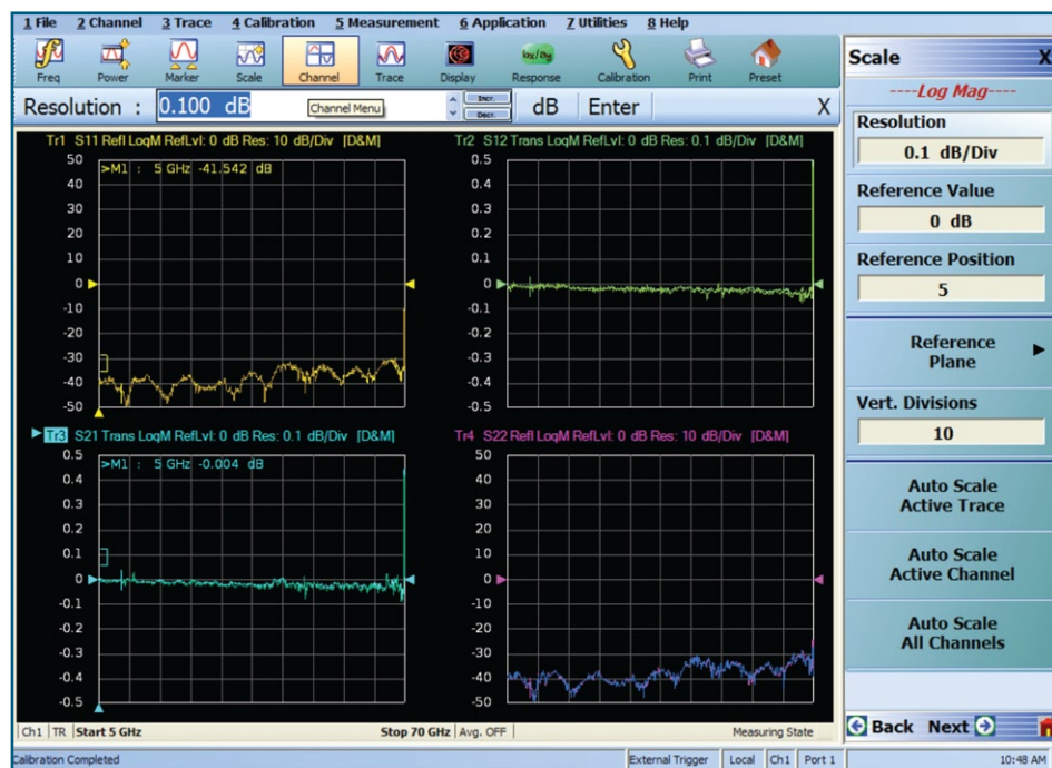
Figure 5: Precision AutoCal measurement of airline transmission; note ability to handle low loss measurement.
